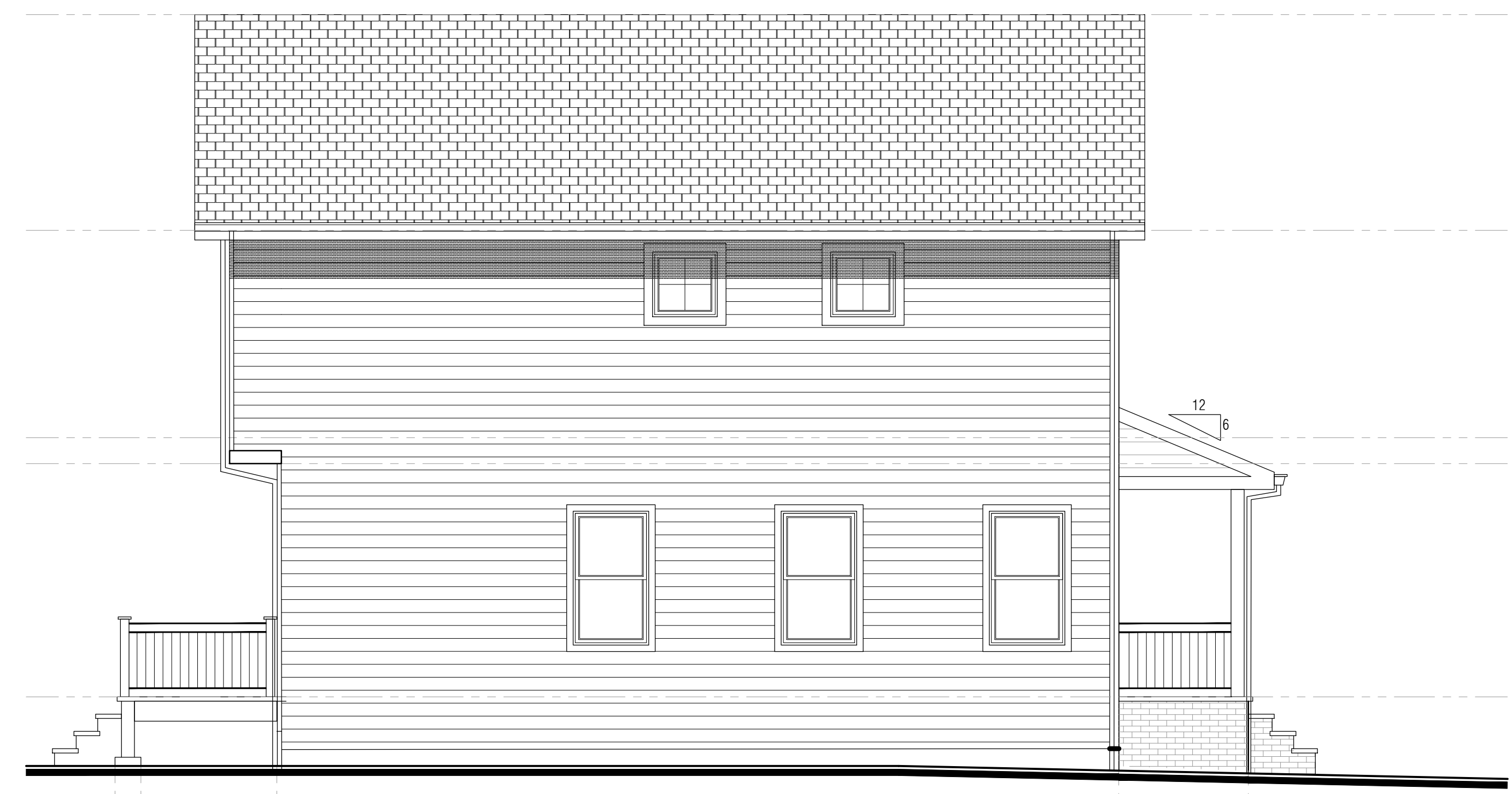
3 PROPOSED SOUTHWEST ELEVATION SCALE: 1/4" = 1'-0"
